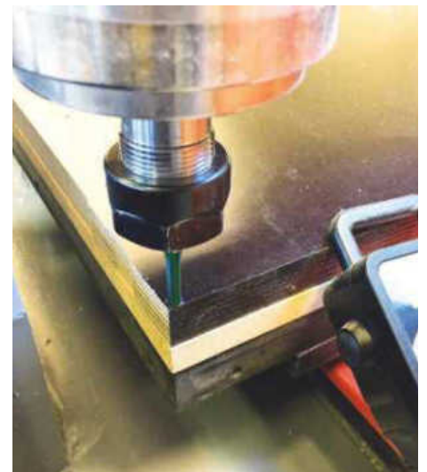
PIC 8. The start-point is zeroed using a remote controller
